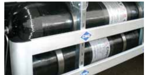
The RCVs have been converted to use natural gas and biomethane as the primary fuel source.
