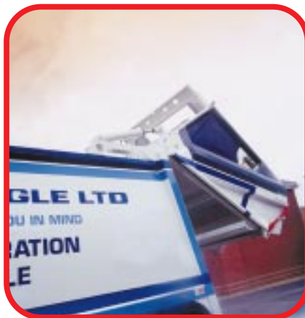
The tailgate design, now fixes to the main body in a 10 degree plane.
